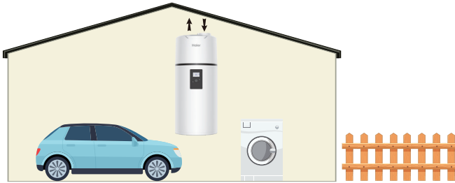
Garage or laundry room (without ducts)
